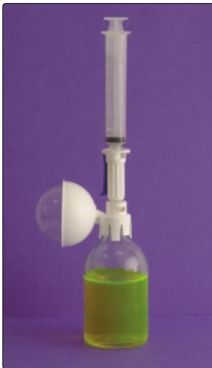
Figure 1. The PhaSeal system attached to a 100 mL vial containing 80 mL fluorescein solution
